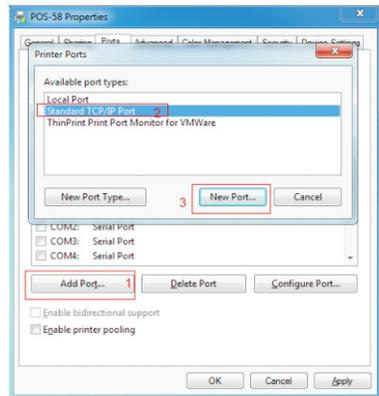
4. According Add Standard TCP / IP Printer Port Wizard, click Next continued following the installation, as shown below:
