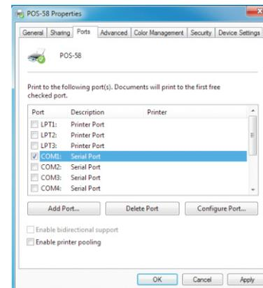
2. Select the list of ports "COM1" → "Configure Port", choose the right option. Here are our default parameter, you can see the parameters of serial port from self-test page
