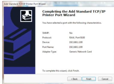
8. Find the printer driver-pos58, Click the "Printer property", and choose the "Ports", select the correct IP port, click "Apply", as shown below:
